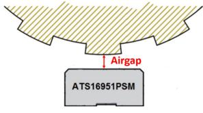
Figure 6: Air gap definition
