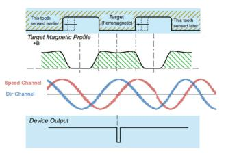
Figure 2: Output in the middle of the tooth
