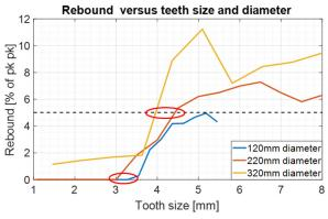
Figure 8: Speed channel 50% rebound level versus tooth size
