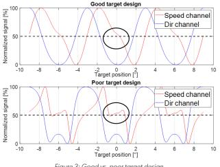
Figure 3: Good vs. poor target design
