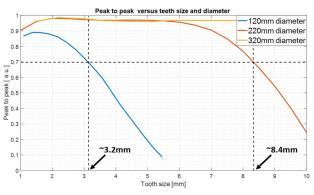
Figure 10: Speed channel peak-to-peak versus teeth size and diameter
