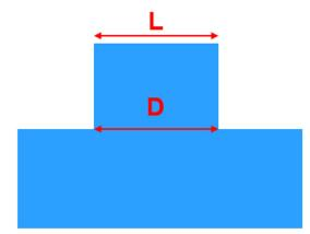
Figure 7: Ratio 1 tooth shape
