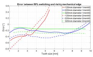
Figure 12: Dir channel rising edge error
