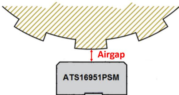
Figure 6: Air gap definition
