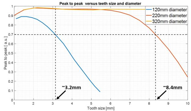
Figure 10: Speed channel peak-to-peak versus teeth size and diameter
