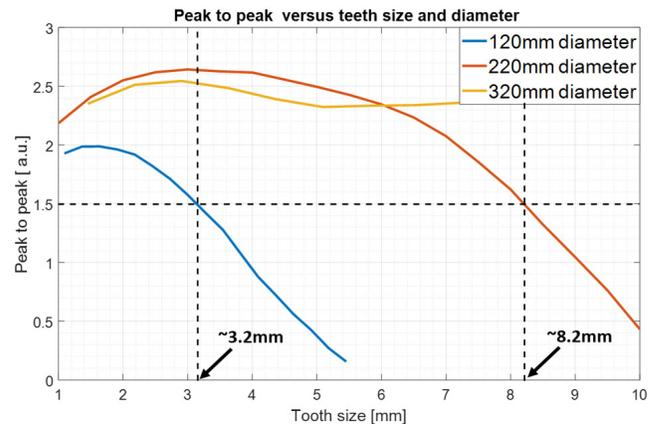
Figure 11: Dir channel peak-to-peak versus tooth size and diameter
