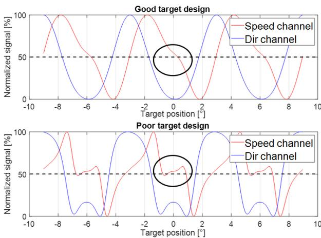
Figure 3: Good vs. poor target design
