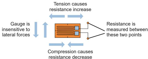
Figure 6: Resistance behavior of strained gauge
