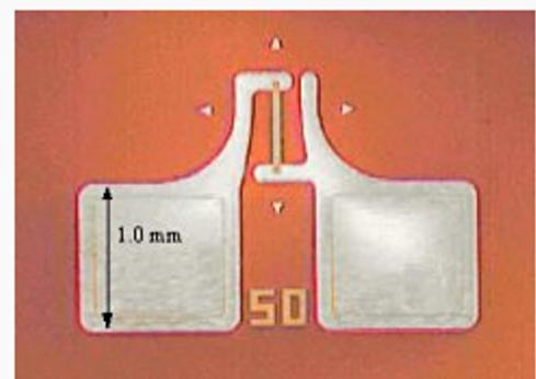
Figure 2: Vertical semiconductor strain gauge between metal pads.
