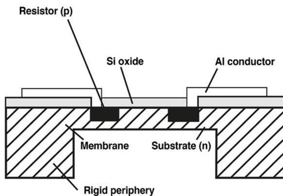
Figure 5: Semiconductor strain gauge
