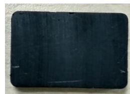
Figure 6: Ferrite Magnet (Size: 27.5 mm × 18 mm × 6 mm)
