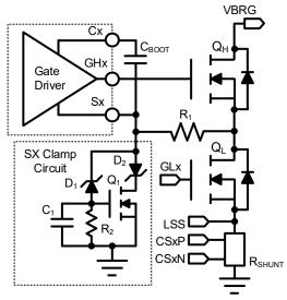
Figure 9 : Gate driver protection circuitry
