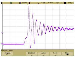
Figure 4: Example of excessive overshoot and ringing
