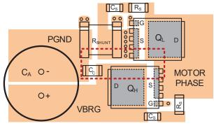
Figure 3: PCB Layout
