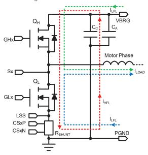
Figure 1: Power section of half-bridge discrete MOSFET design
