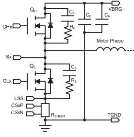
Figure 2 : Bridge Circuit Layout
