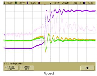
Figure 8 provides some additional insight on the effect of using series gate resistors. The yellow and green traces are the gate and source of the low side MOSFET, and the pink
