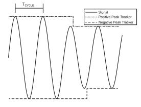
Figure 1: Peak Tracking Example
