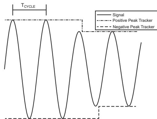
Figure 1: Peak Tracking Example
