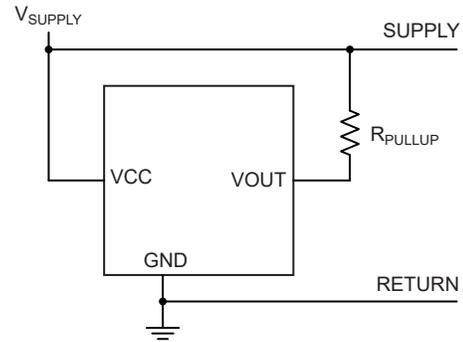
Figure 8: Conversion of three-wire to two-wire
