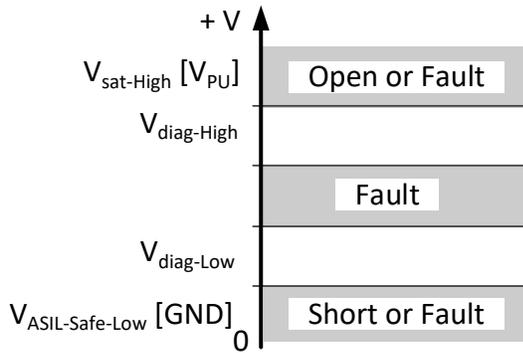
Figure 7: Three-wire output states including diagnostic
