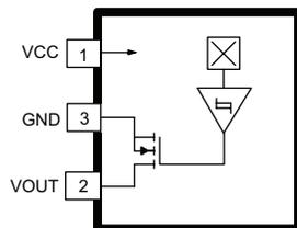
Figure 1: Example three-wire IC pinout
