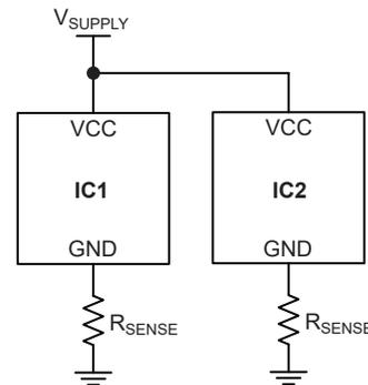
Figure 9: Two two-wire ICs on shared supply
