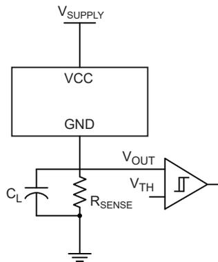
Figure 5: Two-wire interface circuit
