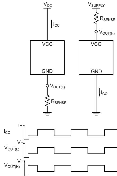
Figure 6: High and low side sensing
