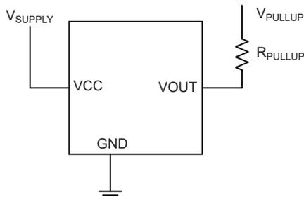
Figure 2: Three-wire interface circuit
