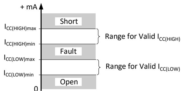
Figure 4: Two wire digital levels
