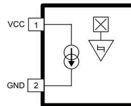
Figure 3: Example two-wire IC pinout
