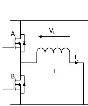
Figure 2: Complementary switching circuit.
