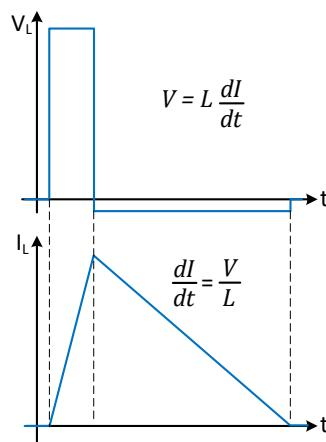
Figure 1: Driving inductive load.
