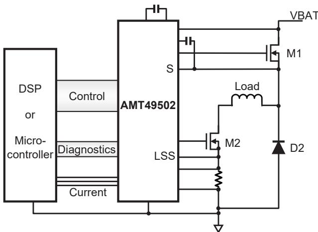
Figure 3: AMT49502 PWM load current control.
