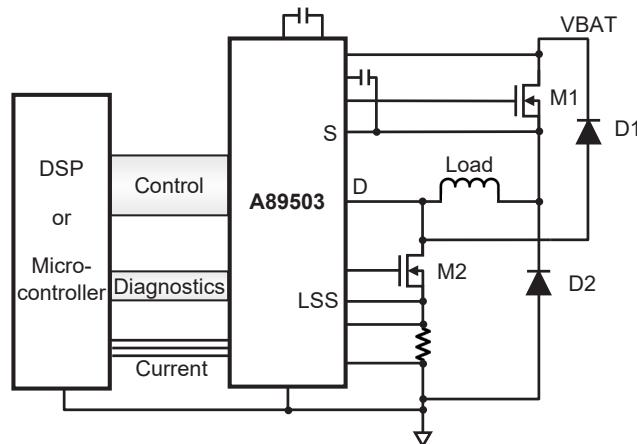
Figure 4: A89503 PWM load current control.
