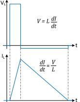
Figure 1: Driving inductive load.
