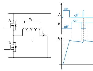
Figure 2: Complementary switching circuit.
