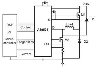
Figure 4: A89503 PWM load current control.
