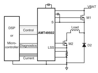
Figure 3: AMT49502 PWM load current control.
