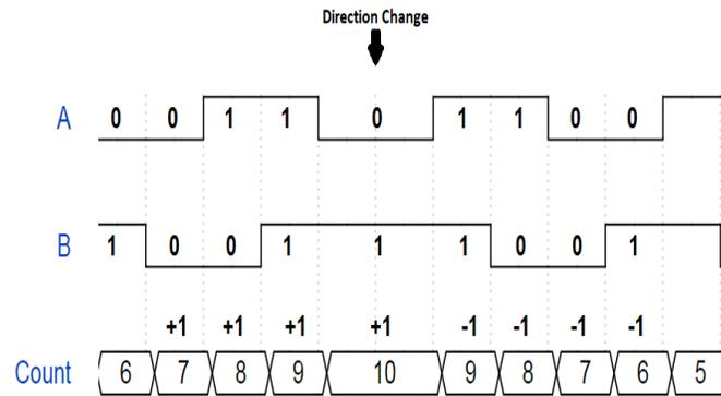
Figure 9: AB protocol encoding state transitions
