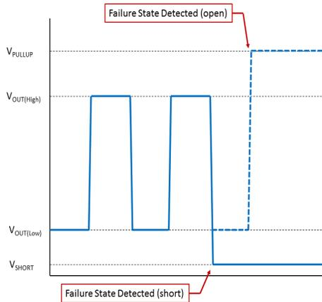
Figure 12: ECU Fault Condition detection
