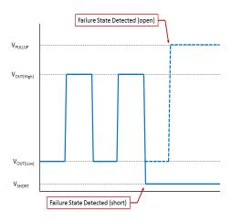
Figure 12: ECU Fault Condition detection
