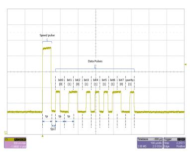
Figure 11: Scope capture of a single AK message showing a speed pulse followed by the data pulses and the decoding of the data pulses to bits
