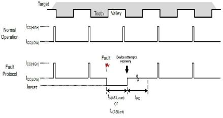
Figure 13: Safe state for 2-wire current interface
