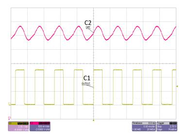
Figure 2: Scope capture of the differential magnetic signal (C2) and the respective speed only output (C1)
