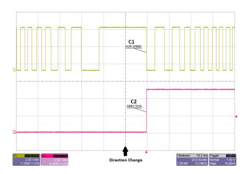
Figure 10: Scope capture of the XOR speed (C1) and DIRECTION (C2) signals during a direction change. Direction is reported on the next edge immediately after direction change
