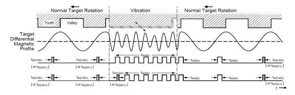
Figure 5: Example output of a device using variable pulse width output during a vibration condition
