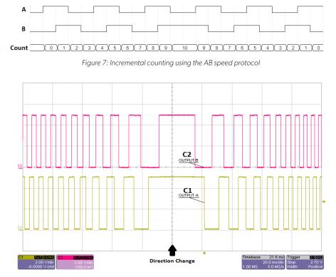
Figure 8: Scope capture of the A and B output signals (C1, C2) from the AB speed protocol during a direction change
