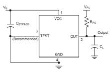
Figure 3: Typical application circuit for an open drain speed-only sensor. Bypass and load capacitors added to meet EMC requirements
