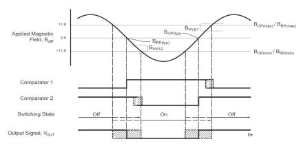
Figure 1: Example of switching scheme for a speed-only sensor
