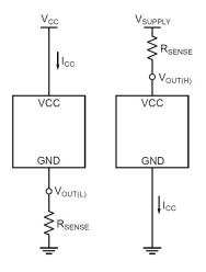
Figure 4: Typical application circuit for a current-interface sensor
