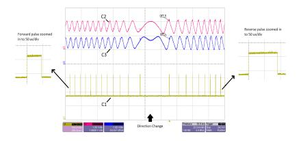
Figure 6: Scope capture of the right and left differential signals (C2, C3) and the respective pulse width output signal (C1) during a direction change from forward rotation to reverse rotation
