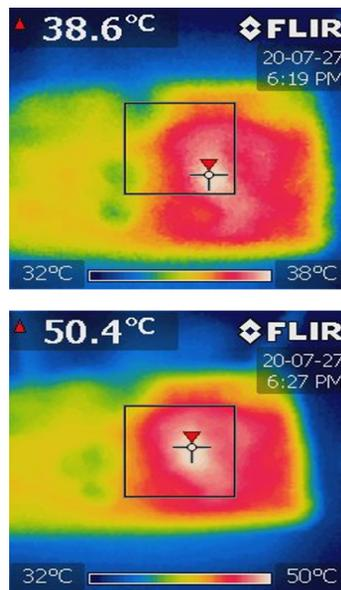
Figure 5: Comparison of steady state temperature increase of the A4480 and a standalone LDO at 12 V, 50 mA current on a 25 mm × 35 mm PCB.
