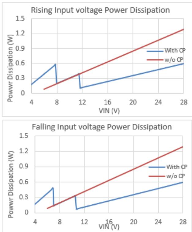
Figure 4: Comparison of steady state power dissipation of the A4480 and a standalone LDO
