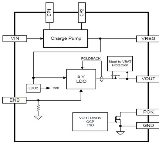
Figure 2: Functional block diagram of the A4480
