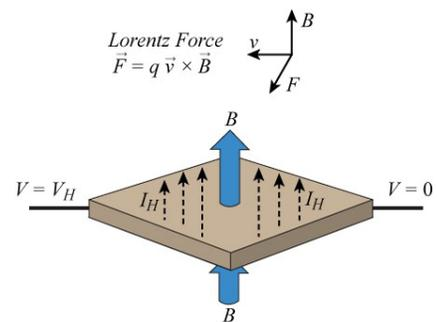
Figure 1: Simplified Hall plate diagram.
