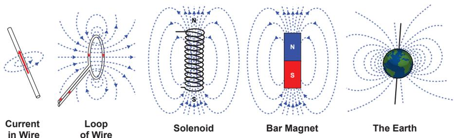
Figure 1: Magnetic Field Sources
