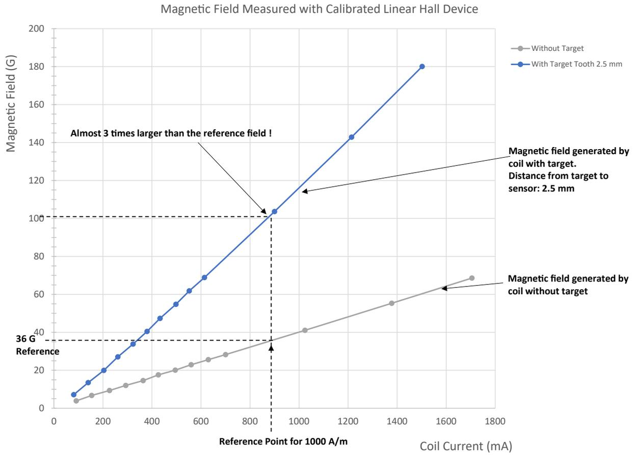
Figure 2: Impact of Ferromagnetic Target in a Helmholtz Coil
