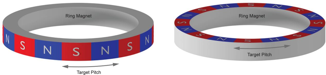
Figure 1: Example of radial (left) and axial (right) ring magnet
