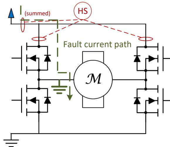
Figure 8: Fault current path using high-side current sensing
