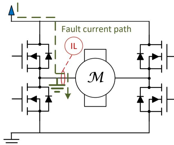
Figure 12: Fault current path using in-line current sensing
