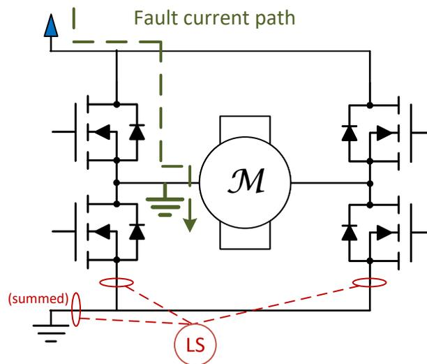
Figure 4: Fault current path using low-side current sensing
