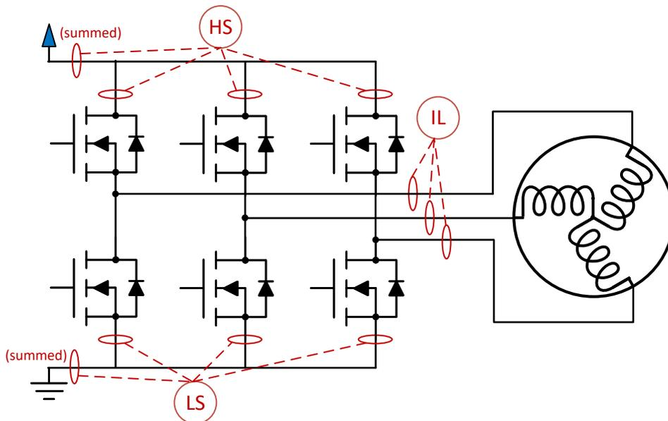
Figure 3: Brushless DC motor driver circuit
