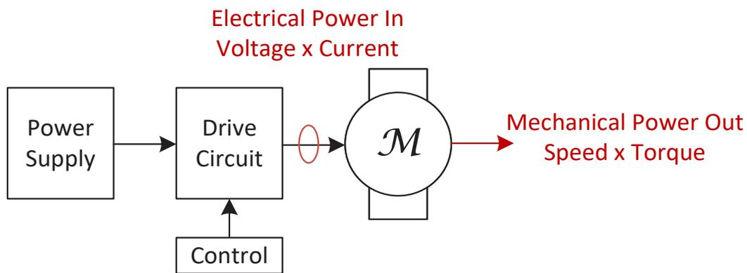
Figure 1: General diagram of current sensing in motors
