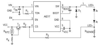
Figure 12: A6217 with Thermal Derating By Control of the Current Sense (CS) Voltage
