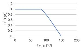
Figure 13: A6217 Thermal Derating, I<sub>OUT</sub> vs. Temperature
