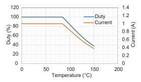
Figure 18: A80804 Thermal Derating Using Internal PWM Dimming Feature
