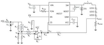
Figure 14: A6217 Buck LED Driver and Op-Amp with LDO for Derating Proportional to Temperature
