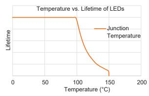
Figure 1: Typical Temperature vs. Lifetime Curve of LED
