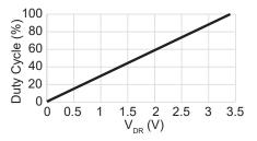
Figure 17: A80804 VDR Pin Voltage vs. Duty Cycle
