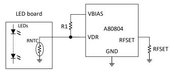
Figure 16: A80804, 100% Duty Cycle During Typical Operation and Thermal Derating Using PWM Dimming
