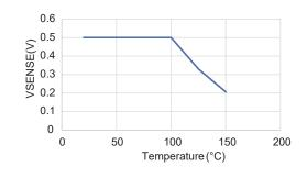
Figure 10: V<sub>SENSE</sub> vs. Temperature
