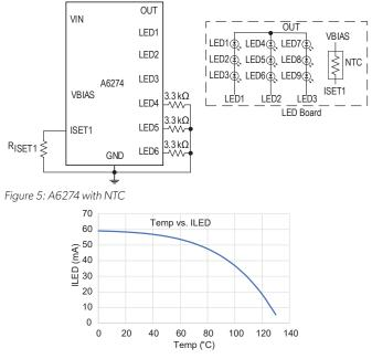
Figure 6: Temperature vs. I<sub>LED</sub>
