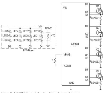
Figure 9: A80804 Thermal Derating Using Analog Dimming
