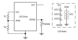
Figure 7: NTC Connection for LED Driver with Separate ADIM Pin
