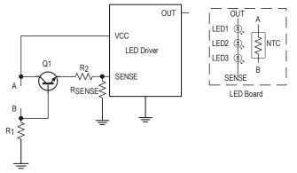
Figure 11: LED Driver with Transistor in Emitter-Follower Configuration and
