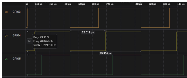
Figure 8: ADC Calibration Trigger on Phase B
