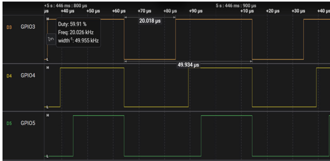
Figure 7: ADC Calibration Trigger on Phase A
