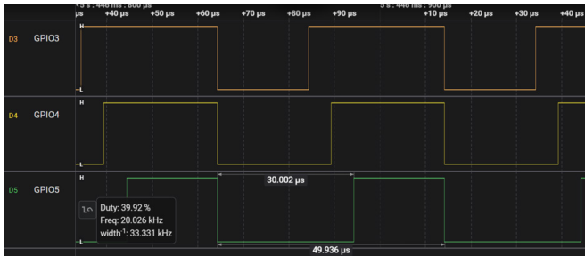
Figure 9: ADC Calibration Trigger on Phase C
