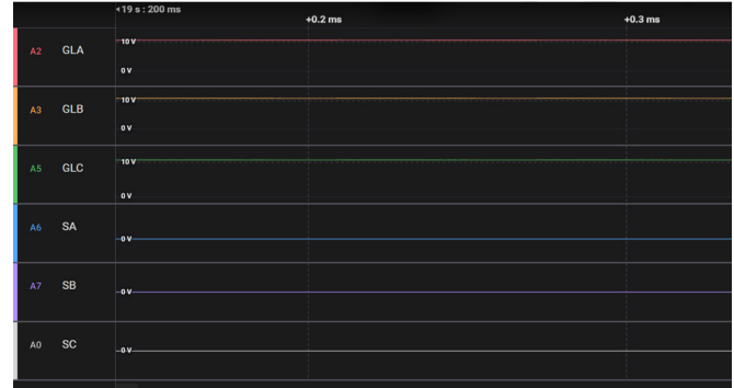
Figure 4: Low-Side On Waveform
