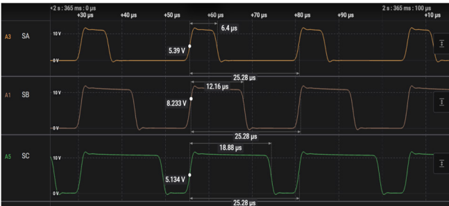
Figure 3: Edge-Aligned Mode Waveform
