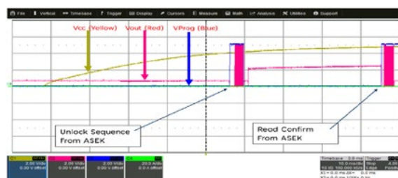
Figure 9: Oscilloscope capture showing Manchester unlock and read confirm following external V CC trigger level.
