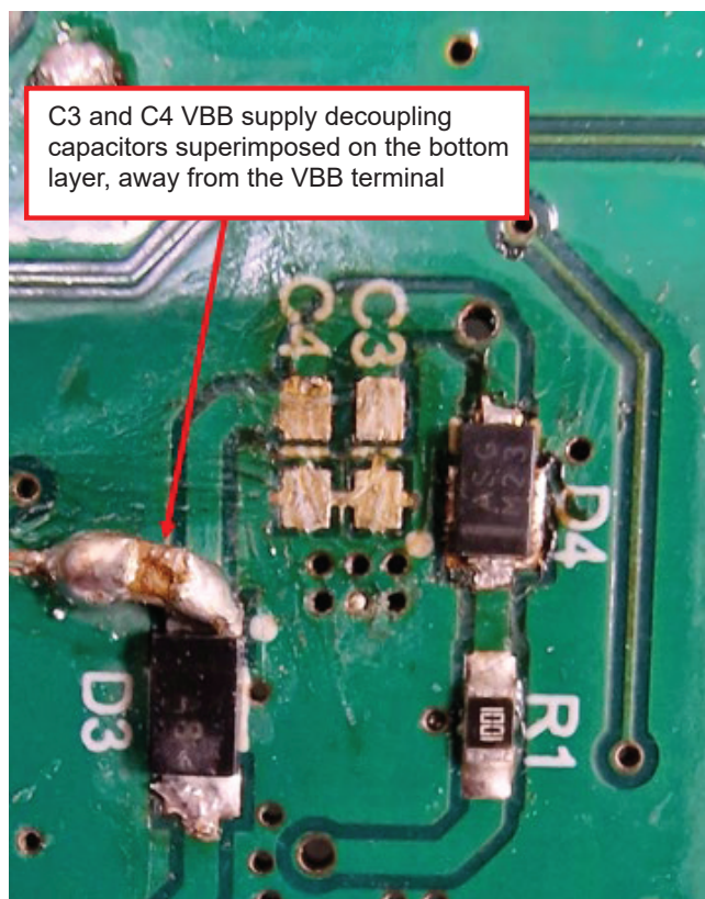
Figure 9: Supply Capacitors Far From VBB, Not Recommended
