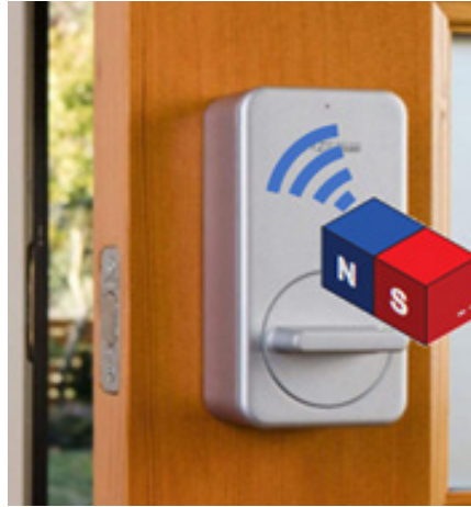
Figure 1: Smart Lock Vulnerability Mechanism
