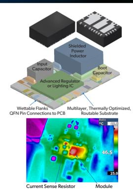
By housing discrete components in clever packaging, ClearPower modules manage heat, speed product design, and achieve 5× less EMI.
