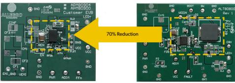
ClearPower LED Driver Module  $10 \text{ mm} \times 14 \text{ mm} = 140 \text{ mm}^2$
