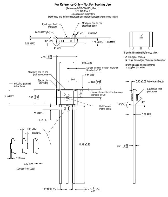
Figure 5: Package UA, 3-Pin SIP
