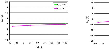
**Operate Point versus Ambient Temperature**
