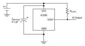
**Figure 2: Typical Application Circuit**
