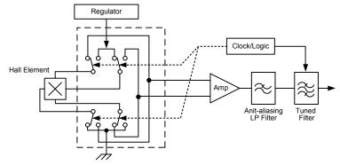
Figure 3: Concept of Chopper Stabilization Technique
