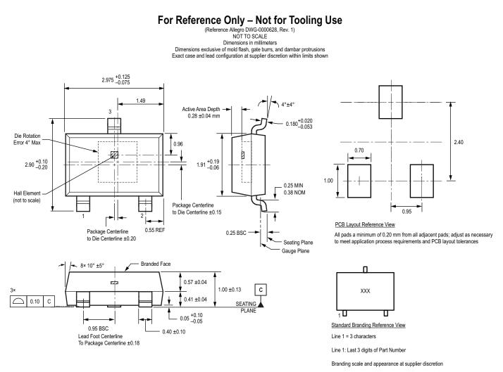
Figure 4: Package LH, 3-Pin SOT23W
