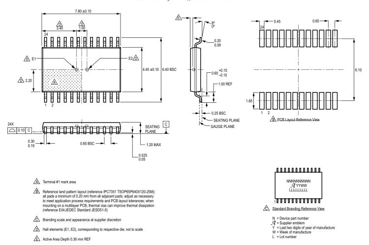
Figure 29: Package LE, 24-Pin TSSOP (Dual-Die Version)
