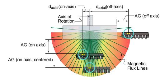
Figure 17: The magnetic flux density degenerates rapidly away from the plane of peak north-south polarity. When the axis of rotation is placed away from the Hall element, the device must be placed closer to the magnetic poles to maintain an adequate level of flux at the Hall element.
