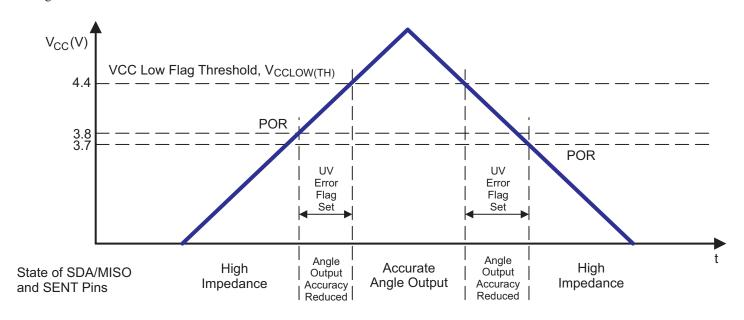
Figure 2: Relationship of V<sub>CC</sub> and Output
