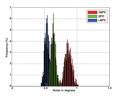
Figure 24: Noise Distribution over Temperature (3 Sigma, 300 G)
