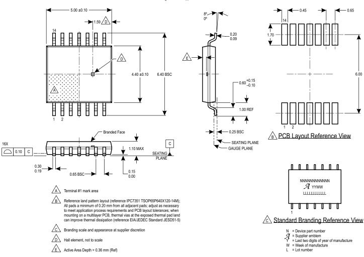
Figure 28: Package LE, 14-Pin TSSOP (Single-Die Version)
