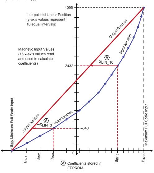
Figure 20: Sample of Linearization Function Transfer Characteristic
