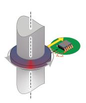
Industry-leading linearization enables off-axis (side-shaft) operation
