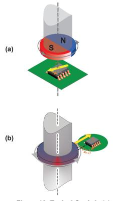
Figure 13: Typical On-Axis (a) and Off-Axis (b) Orientation
