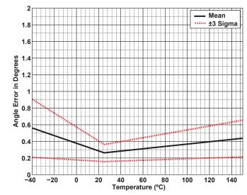
Figure 22: Peak Angle Error over Temperature (300 G)
