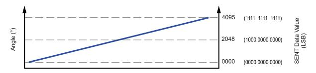
Figure 4: Angle is Represented as a 12-bit Digital Value
