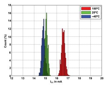
Figure 26:  $I_{CC}$  Distribution over Temperature  $(V_{CC} = 5.5 \text{ V})$
