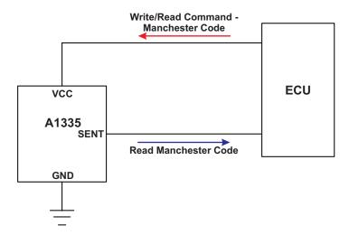
Figure 3: Top-Level Programming Interface
