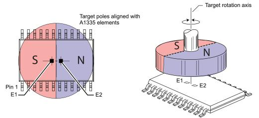
Figure 12: Orientation of Magnet Relative to Primary Die and Secondary Die
