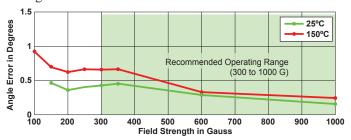
Figure 9: Typical Maximum Angle Error
