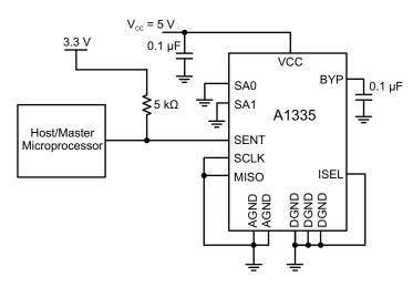
(C) Typical A1335 configuration using SENT interface (SA0/SA1 may be brought to BYP or GND to configure Manchester/Shared SENT address)
