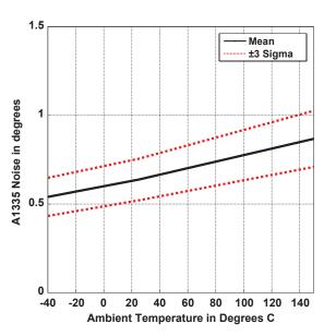
Figure 25: Noise Performance over Temperature (3 Sigma, 300 G)
