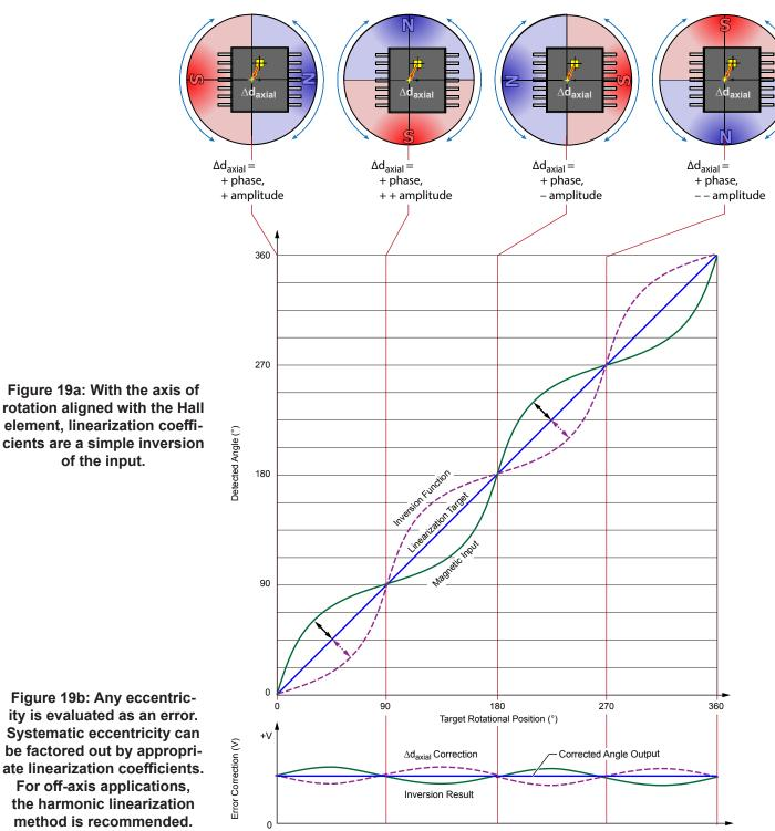
ity is evaluated as an error. Systematic eccentricity can be factored out by appropriate linearization coefficients. For off-axis applications, the harmonic linearization
