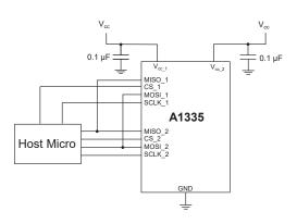
Figure 30: Separate SCLK Lines
