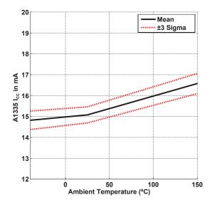
Figure 27:  $I_{CC}$  over Temperature  $(V_{CC} = 5.5 \text{ V})$
