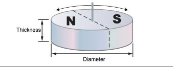
[1] A sintered neodymium magnet with 10 mm (or greater) diameter and 4 mm thickness is the recommended magnet for redundant applications.
