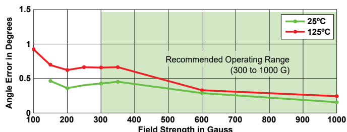
Figure 14: Typical Maximum Angle Error Over Field Strength
