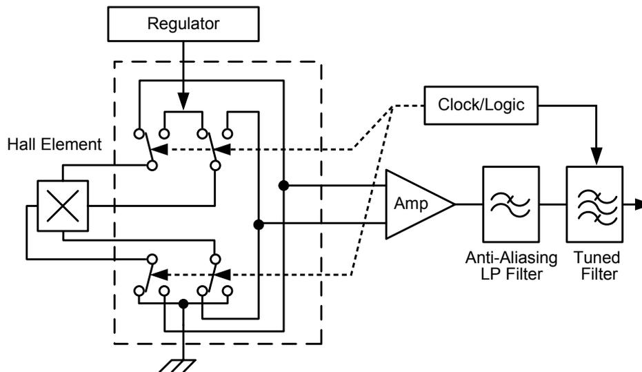
Figure 8: Concept of Chopper Stabilization
