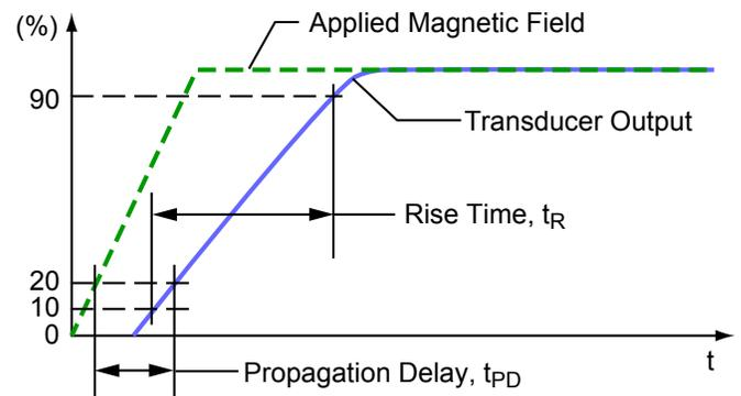
Figure 2: Propagation Delay and Rise Time definitions
