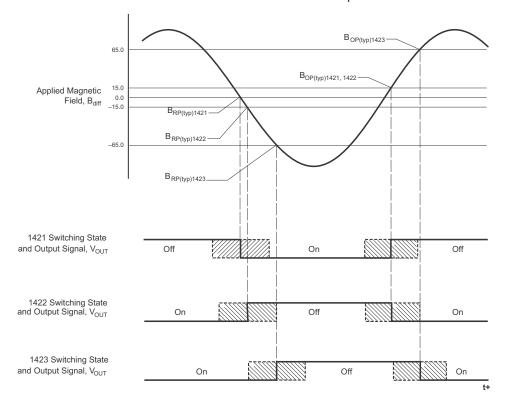
Figure 2. Comparative typical output characteristics. This chart illustrates the switch points and the output polarities of the A1421, A1422, and the A 1423. Characteristics shown without delay, see characteristic data charts for delay and phase shift contributions.
