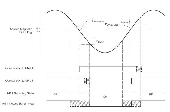
Figure 1. Typical output characteristics with dual comparator operation. The example shown is for the A1421. Characteristics shown without delay, see characteristic data charts for delay and phase shift contributions.
