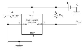
Figure 3. Basic application circuit. A pull-up resistor,  $R_{\text{PU}}$ , is required with the output driver.
