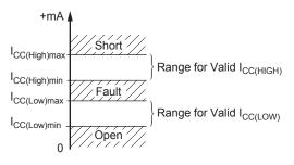
Figure 8: Diagnostic Characteristics of Supply Current Values
