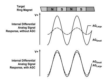
Figure 5. Automatic Gain Control (AGC). The AGC function corrects for variances in the air gap. Differences in the air gap affect the magnetic gradient, but AGC prevents that from affecting device performance, as shown in the lowest panel.
