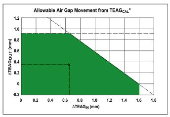
\*Data based on study performed using spur gear reference target 60-0, and applicable to ring magnet targets with similar magnetic characteristics.
