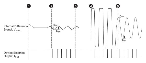
Figure 9: Operation of Running Mode Gain Adjust.
