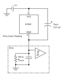
Figure 7: Typical Application Circuit
