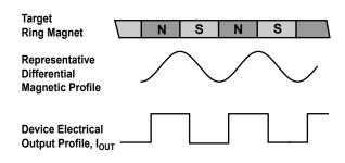
Figure 3. Output Profile of a ring magnet target for the polarity indicated in figure 2.
