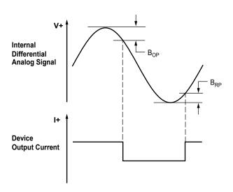
Figure 6: Peak Detecting Switch Point Detail
