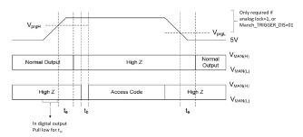
Figure 15: Access Code Write Timing Diagram
