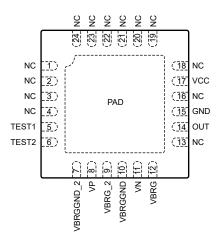
Package ES, 24-Pin QFN Pinout Diagram
