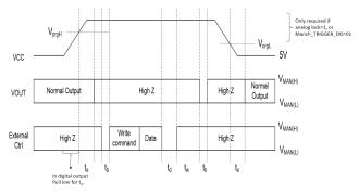
Figure 17: Write to Non-Volatile Memory (EEPROM) Timing Diagram
