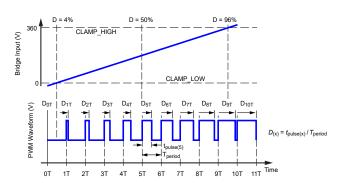
Figure 8: PWM Output Mode - Duty-Cycle-Based Waveform
