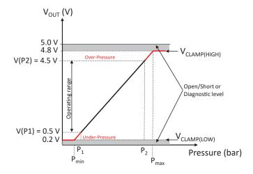
Figure 7: Output Level and Diagnostic Description
