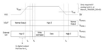
Figure 16: Write to Volatile Memory Timing Diagram
