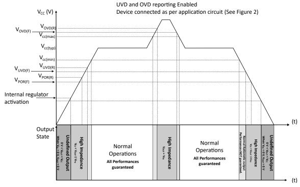
Figure 3: Output Behavior Under  $V_{CC}$  Ramp Conditions
