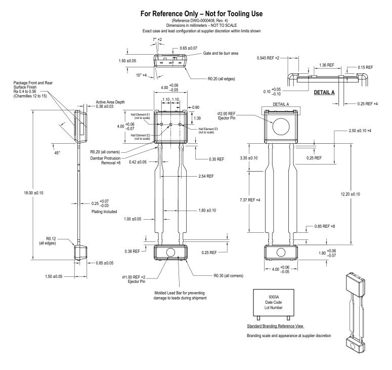
Figure 14: Package UB, 2-Pin SIP
