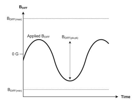
Figure 6: Definition of Differential Magnetic Input
