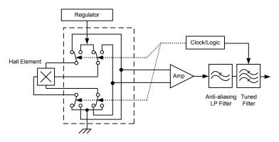
Figure 6. Chopper Stabilization Technique
