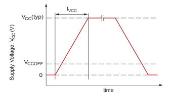
Figure 4. Definition of V<sub>CC</sub> Ramp Time, t<sub>VCC</sub>
