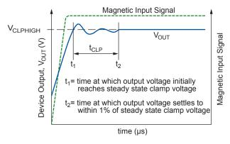
Figure 2. Definition of Delay to Clamp,  $t_{\text{CLP}}$
