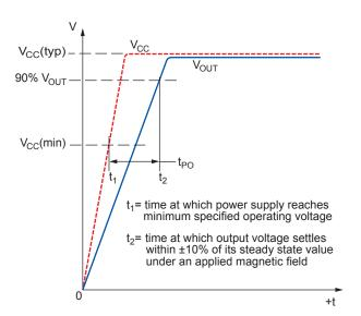
Figure 1. Definition of Power On Time,  $t_{PO}$
