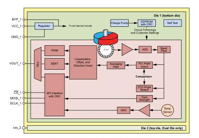
Figure 1: A33002 Magnetic Circuit and IC Diagram
