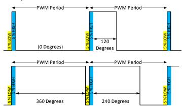
Figure 5: Pulse-Width Modulation (PWM) Examples
