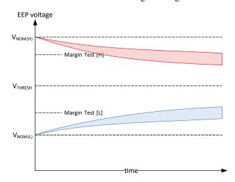
Figure 31: Example of passing programming voltages
