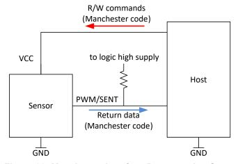
Figure 23: Manchester Interface Programming Setup
