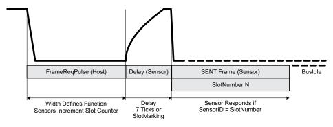
Figure 47: SSENT Sensor Addressing
