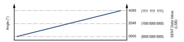
Figure 35: Angle is Represented as a 12-bit Digital Value
