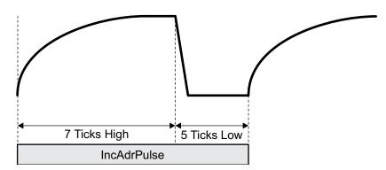
Figure 50: ASENT Incremental Address Pulse (IncAdrPulse) (Output by Host)
