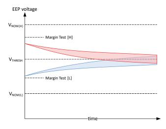
Figure 32: Example of failing programming voltages
