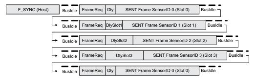
Figure 49: SSENT Sensor Addressing—With Slot Marking (Four Sensors on Bus)
