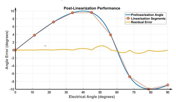
Figure 8: Post-Linearization Error
