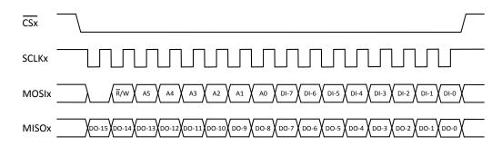
Figure 17: Sixteen-Bit SPI Transaction
