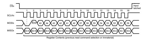
Figure 19: SPI Write Example
