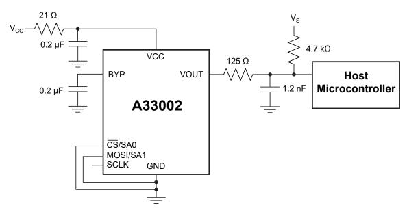
Figure 2: A33002 Reference Design for Stringent EMC Requirements
