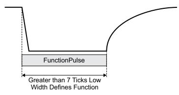
Figure 46: Function Pulse (Output by Host)
