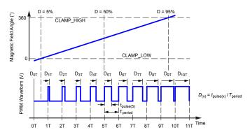
Figure 4: PWM Mode Outputs a Duty Cycle Proportional to Sensed Angle
