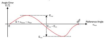
Figure 55: Angle Error Definition
