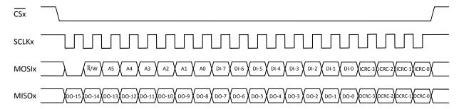
Figure 18: Twenty-Bit SPI Transaction
