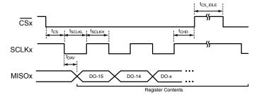
Figure 16: A33002 SPI Interface Timings Output
