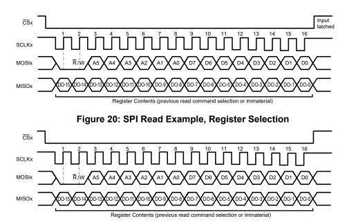
Figure 21: SPI Read Example, Data Output From Selected Register
