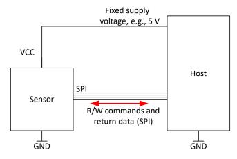
Figure 14: SPI Interface Programming Setup
