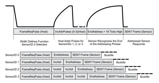
Figure 51: ASENT Sensor Addressing
