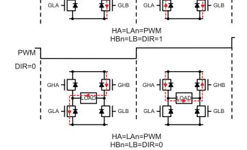
Figure 8: PWM and DIR Inputs, Slow Decay, SR
