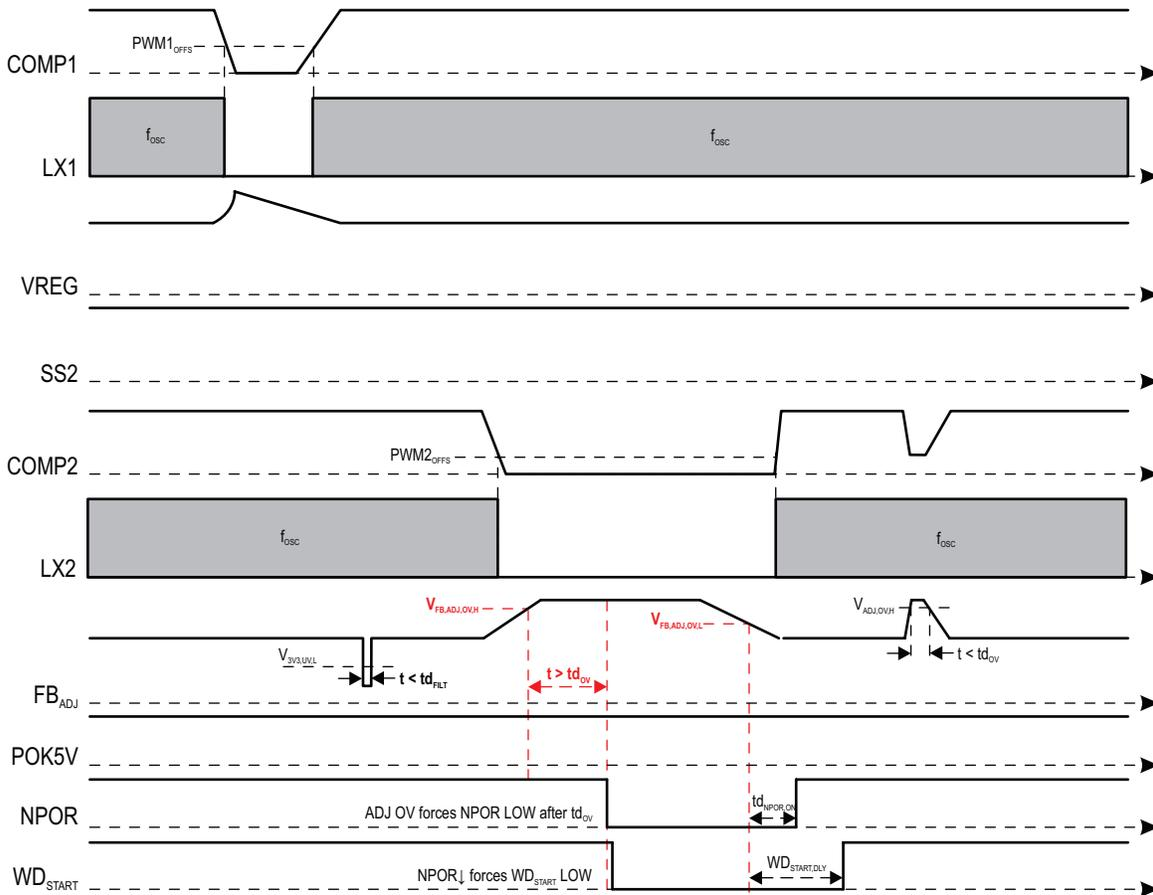
**Figure 14: VREG and FB<sub>ADJ</sub> Overvoltage Operation**
