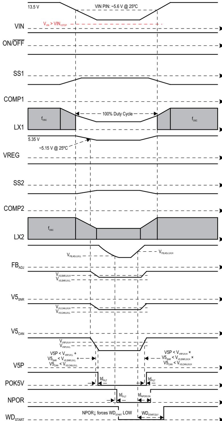
Figure 12: Input Voltage (VIN) Undervoltage,  $V_{VIN} > V_{VIN\_STOP}$
