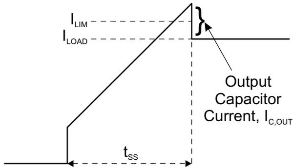
**Figure 19: Output Current ( $I_{CO}$ ) During Startup**
