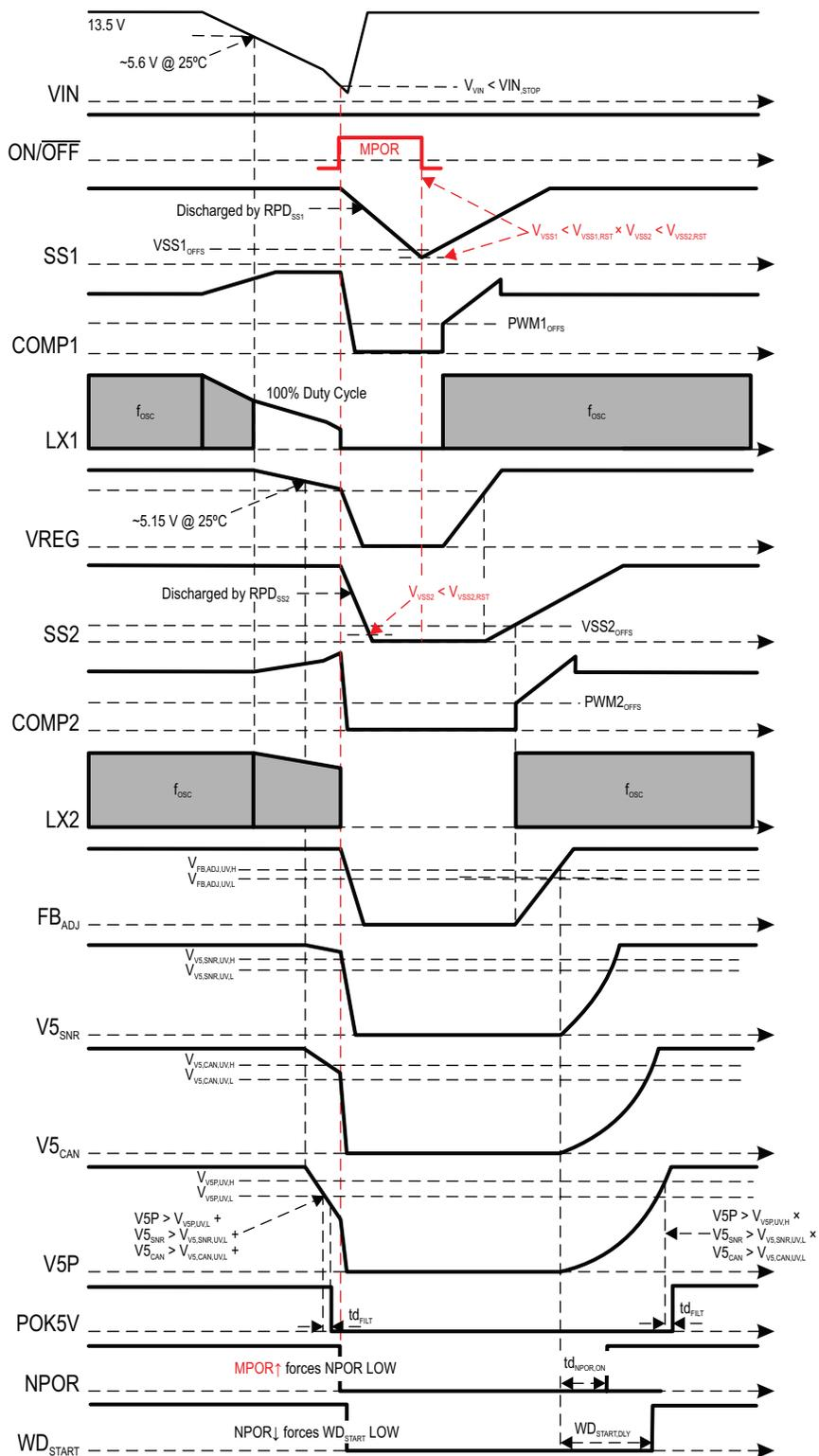
Figure 13: Input Voltage (VIN) Undervoltage,  $V_{VIN} < V_{VIN\_STOP}$
