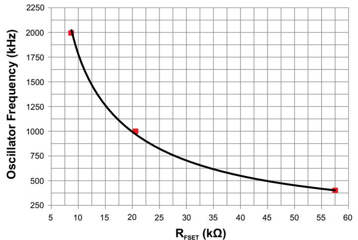
**Figure 8: Switching Frequency vs. FSET Resistor Values**
