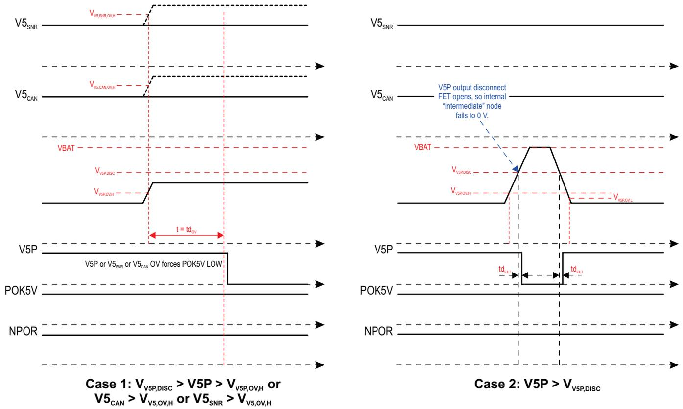
Figure 15: Overvoltage Cases for V5P, V5<sub>SNR</sub>, and V5<sub>CAN</sub>
