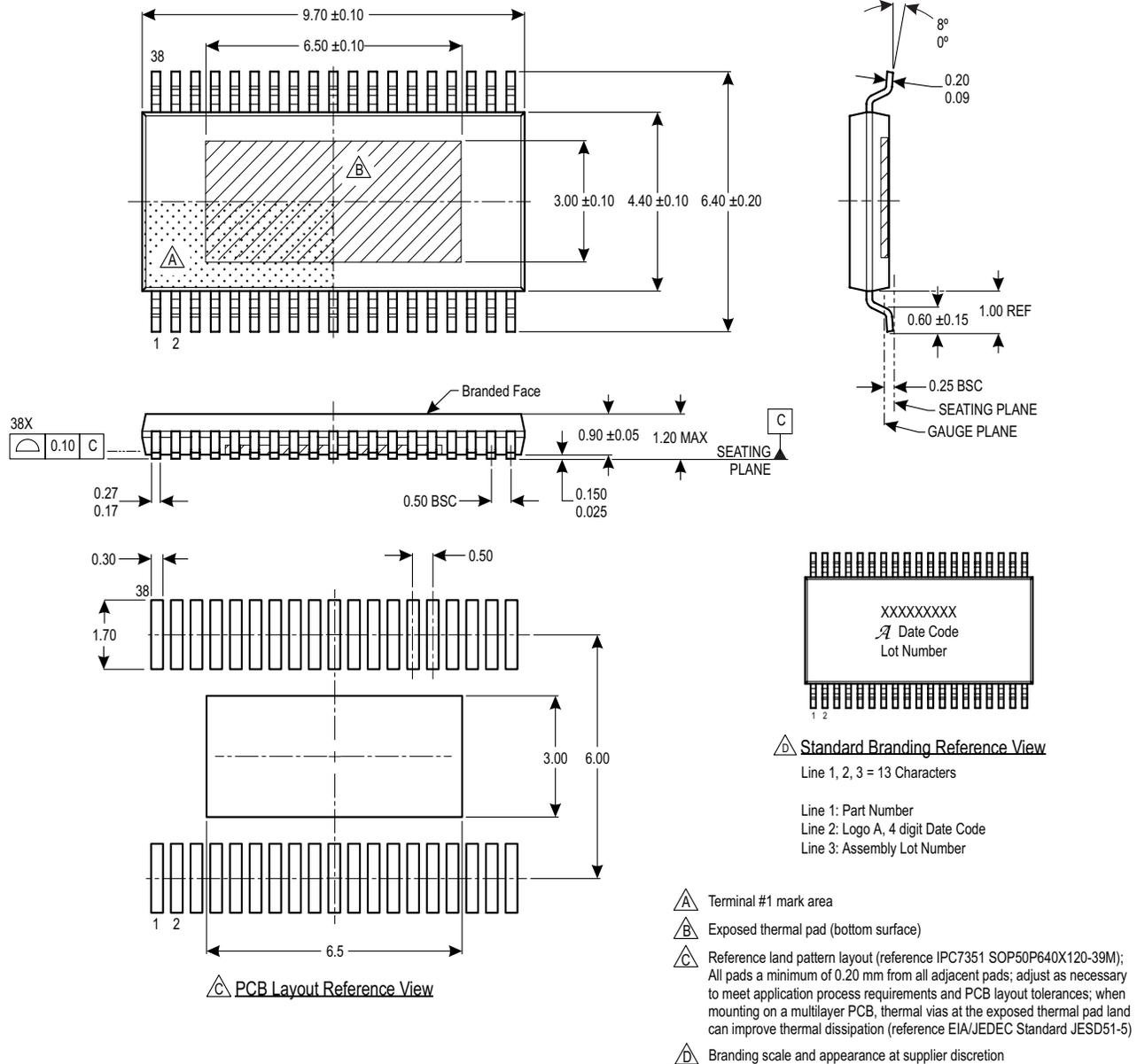
Figure 35: Package LV, 38-Pin eTSSOP
