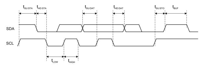
Figure 8: I<sup>2</sup>C-Compatible Timing Requirements
