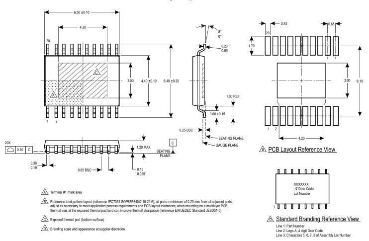
Figure 13: Package LP, 20-Lead TSSOP with Exposed Pad
