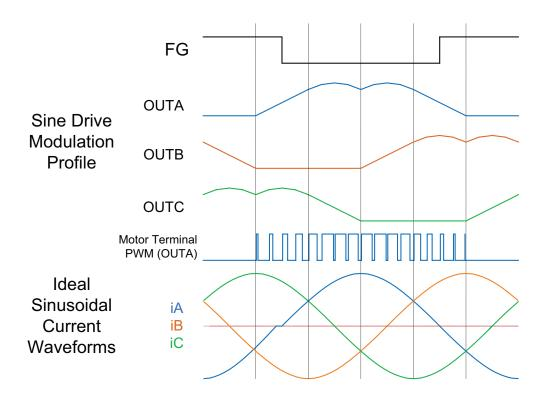
Figure 2: Sinusoidal Drive Sequence
