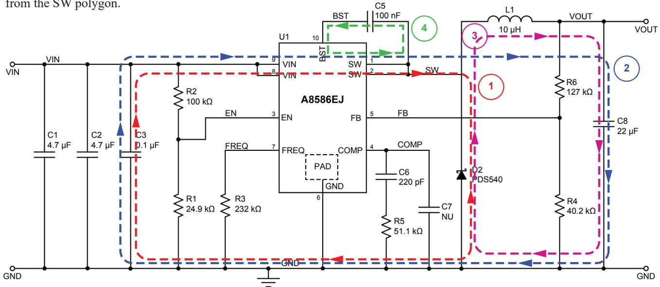
Figure 5: Typical Buck Converter with Critical Paths/Loops Shown
