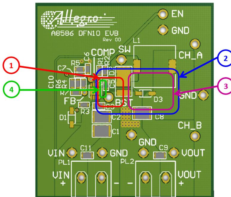
Figure 6: Example PCB Component Placement and Routing
