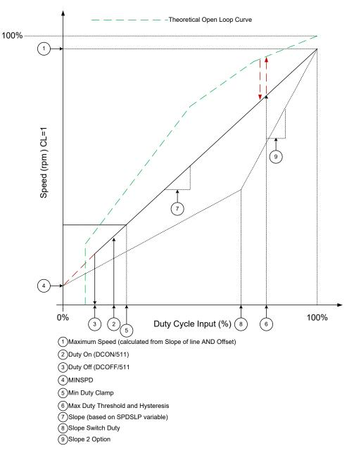
Figure 5: Speed Curve Parameters
