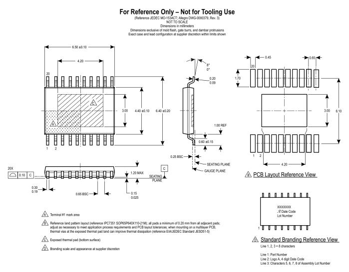
Figure 16: LP Package, 20-Pin TSSOP with Exposed Pad
