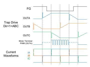
Figure 2: Trapezoidal Drive Sequence for DIR = HI
