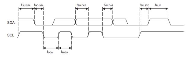
Figure 12: I<sup>2</sup>C-Compatible Timing Requirements
