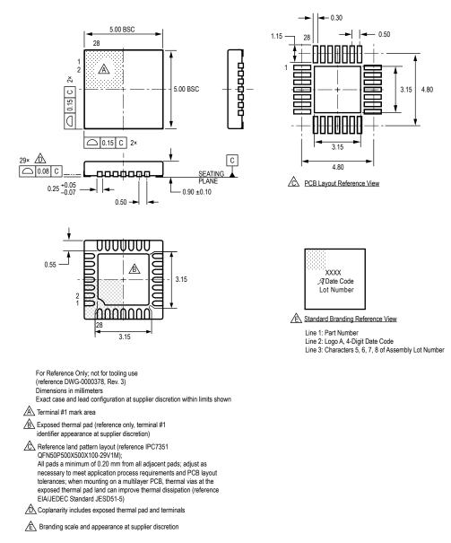
Figure 15: ET Package, 28-Pin QFN with Exposed Pad
