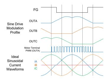
Figure 1: Sinusoidal Drive Sequence for DIR = HI
