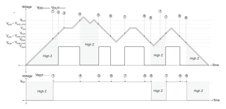
Figure 5: Power States Thresholds with  $V_{OUT}$  Behavior for a 5 V Device,  $R_{L\_VOUT}$  = Pull-Down, UVD Enabled
