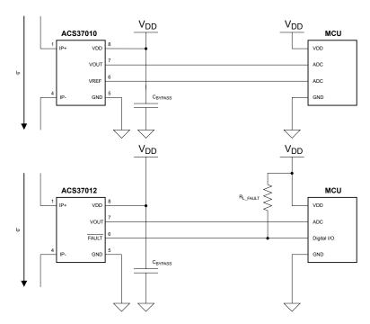
**Figure 1: Typical Application Circuit**
