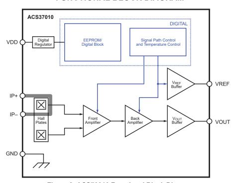
Figure 2: ACS70310 Functional Block Diagram
