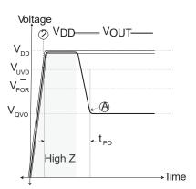
Figure 7:  $t_{PO}$  behavior UVD enabled,  $R_{L VOUT}$  = Pull-Up
