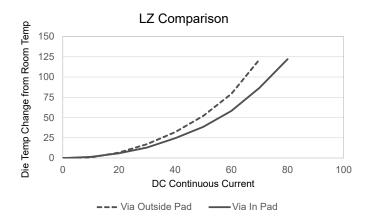
Figure 14: LZ Package Comparison with and without In-Pad Vias
