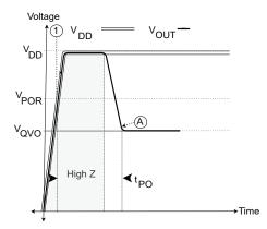
Figure 8:  $t_{PO}$  behavior UVD disabled,  $R_{L VOUT}$  = Pull-Up
