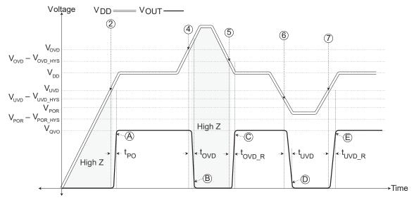
Figure 9:  $t_{PO}$ , and  $t_{OVD}/t_{OVD}$  R, and  $t_{UVD}/t_{UVD}$  R with R<sub>L VOUT</sub> = Pull-Up
