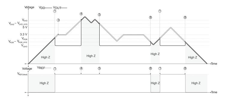
Figure 6: Power States Thresholds with  $V_{OUT}$  and  $V_{REF}$  Behavior, 3.3 V Device,  $R_L$  = Pull-Up, UVD Disabled
