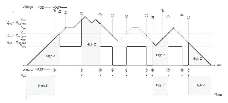
Figure 4: Power States Thresholds with  $V_{OUT}$  and  $V_{REF}$  Behavior, 5 V Device,  $R_{L\_VOUT}$  = Pull-Up, UVD Enabled
