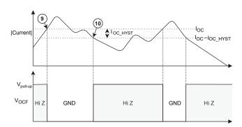
Figure 10: Fault Thresholds and OCF Pin Functionality
