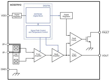
Figure 3: ACS37012 Functional Block Diagram
