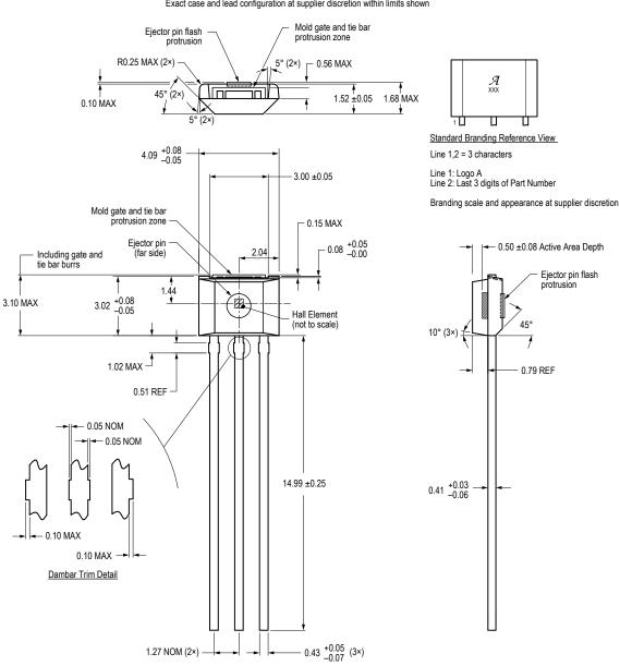
Figure 15: Package UA, 3-Pin SIP
