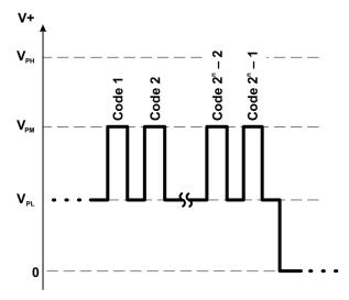
Figure 7: Try Mode Bit Field Addressing Pulse Train
