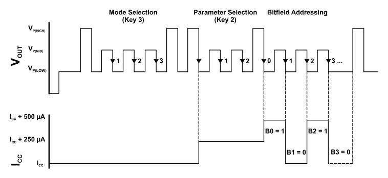
Figure 11: Example of Read Mode Programming Pulses Applied to the VOUT Pin and Device Response in I<sub>CC</sub>.
