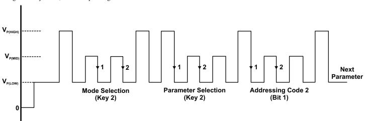
Figure 10: Example of Try Mode Programming Pulses Applied to the VOUT Pin.
