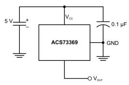
**Figure 4: Typical Application Circuit**
