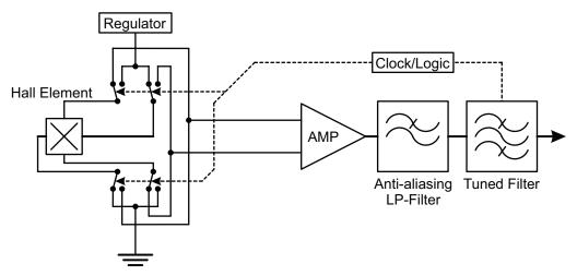
Figure 5: Concept of Chopper Stabilization Technique
