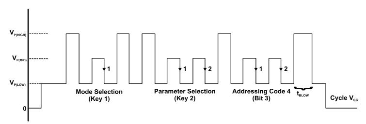
Figure 9: Example of Blow Mode Programming Pulses Applied to the VOUT Pin.
