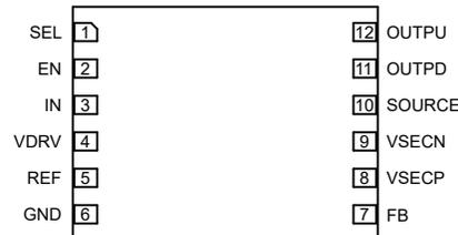
Package NH Pinout (Top View)
