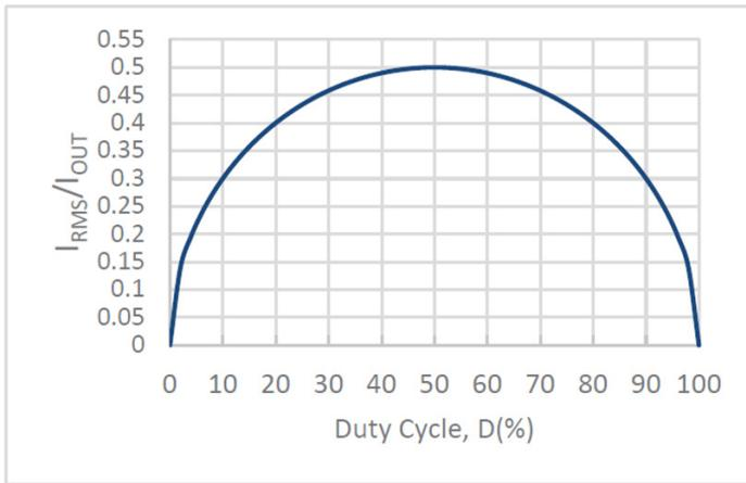
**Figure 10: Normalized Input Capacitor Ripple versus Duty Cycle**
