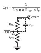
Figure 12: Feedback Divider with Feedforward Capacitor
