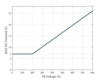
Figure 6: BIAS Overvoltage Threshold vs. FB Pin Voltage
