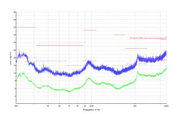
Radiated Emissions (30 MHz to 330 MHz) (Horizontal Biconical)
