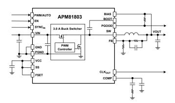
Figure 1: APM81803 Typical Application Circuit
