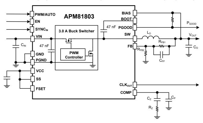
Figure 13: Applications Schematic showing component locations
