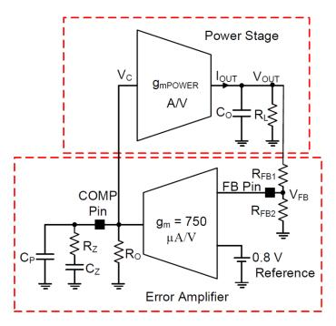
Figure 11: Power Stage and Error Amplifier
