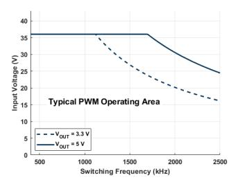
Figure 8: Input Voltage Limit To Prevent Pulse Skipping
