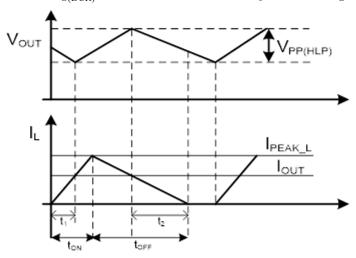
Figure 9: Output Voltage Ripple in LP Mode
