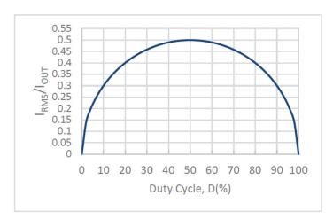
Figure 10: Normalized Input Capacitor Ripple versus Duty Cycle
