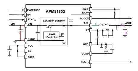
Figure 14: PCB Layout Critical Paths
