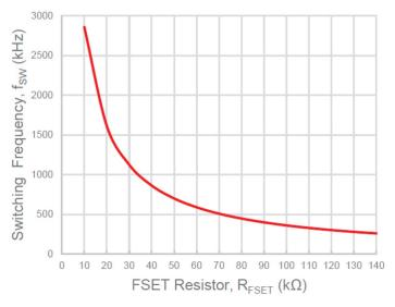
Figure 7: PWM Switching Frequency vs. R<sub>FSET</sub>
