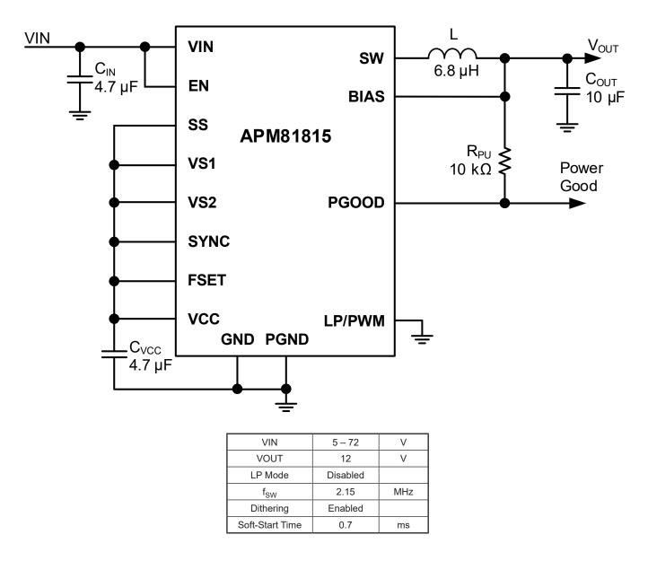
Figure 12: Application Circuit
