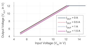
Figure 9: 12 V Output Voltage Dropout at Low V<sub>IN</sub>
