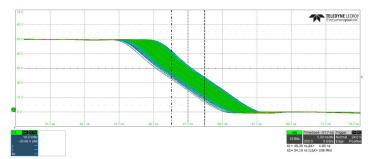
Figure 5: Pulse-Width Jitter with Dither Off, 48  $\rm V_{IN},$  5  $\rm V_{OUT},$  2.2 MHz at 1 A Load
