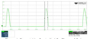
Figure 4: Repeatable, Controlled On-Times of Only 36 ns, 48 V<sub>IN</sub>, 3.3 V<sub>OUT</sub>, 2.2 MHz at 400 mA Load
