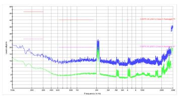
Radiated Emissions (150 kHz to 30 MHz) (Monopole)
