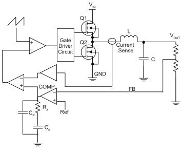
Figure 6:Typical Block Diagram of Average-Current Control Mode
