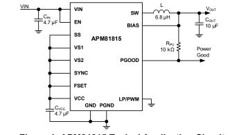
Figure 1: APM81815 Typical Application Circuit
