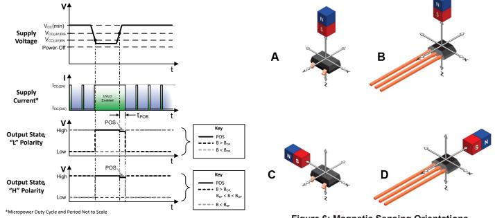
Figure 5: Undervoltage Lockout Behavior
