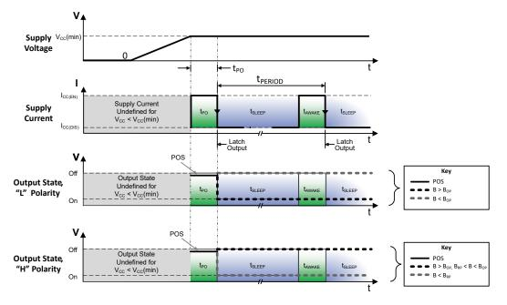
Figure 4: Micropower Operation and Power-On Behavior
