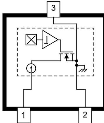
LH Package, 3-Pin SOT23W Pinout
