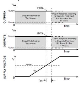
Figure 12: Power-On Sequence and Timing
