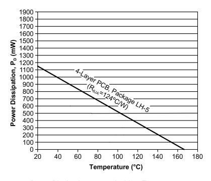
**Power Dissipation versus Ambient Temperature**
