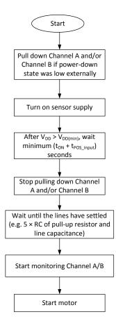
Figure 14: Output setting at power-on, dual quadrature outputs
