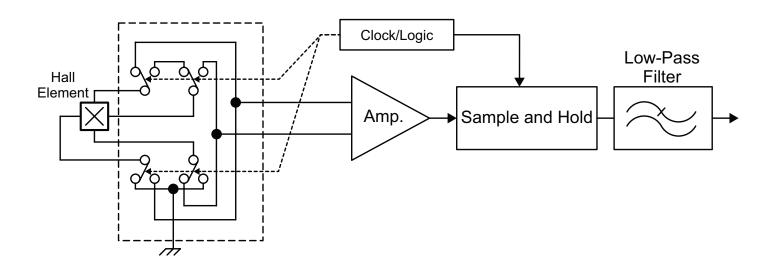
Figure 17: Model of Chopper Stabilization Technique
