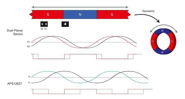
Figure 7: Ring magnet not optimized for a dual-planar Hall-effect sensor resulting in significantly reduced output phase separation, however still results in quadrature for the APS12627/8.
