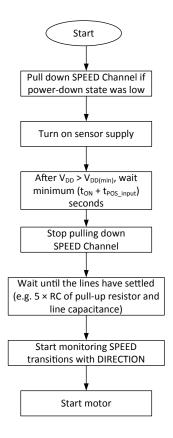
Figure 15: Output setting at power-on, Speed and Direction
