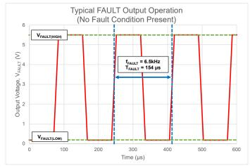
Figure 4: Fault Pin Output - No Fault Present
