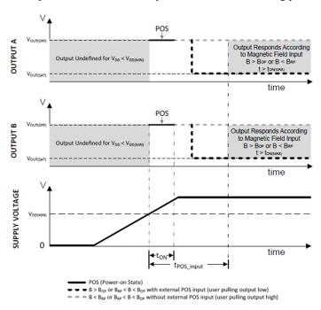
Figure 13: Power-On Sequence and Timing, -P option
