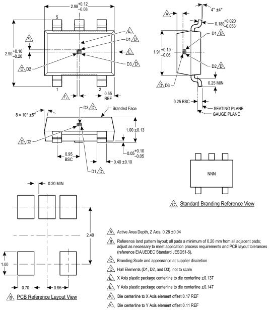
Figure 18: Package LH, 5-Pin SOT23-W
