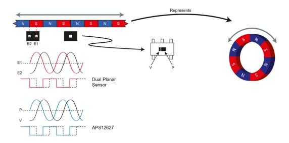
Figure 6: Ring magnet optimized for a dual-planar Hall-effect sensor resulting in output quadrature also results in quadrature for the APS12627/8.
