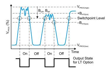
Figure 3: Switch points with Internal Hysteresis
