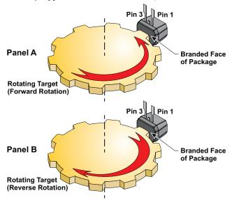
Figure 4: Target Rotation (F Variant Shown)
