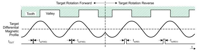
Figure 9: Running Mode Direction Change (-FSxxHxx Variant)
