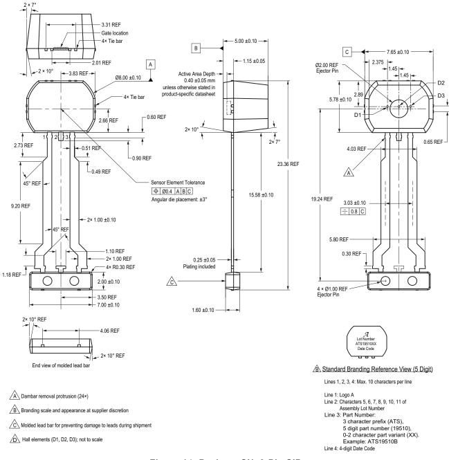
Figure 14: Package SN, 3-Pin SIP
