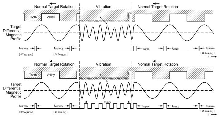
Figure 13: Output Functionality in the Presence of Running Mode Target Vibration (-xxxxHxx Variant)
