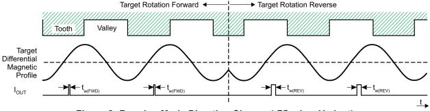
Figure 8: Running Mode Direction Change (-FSxxLxx Variant)
