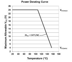
A worst-case estimate,  $P_{D(max)}$ , represents the maximum allowable power level ( $V_{CC(max)}$ ,  $I_{CC(max)}$ ), without exceeding  $T_{J(max)}$ , at a selected  $R_{\theta JA}$  and  $T_A$
