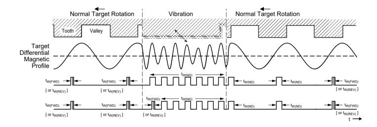
Figure 7: Output protocol options with non-direction pulses
