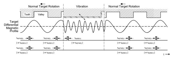
Figure 6: Vibration output protocol options
