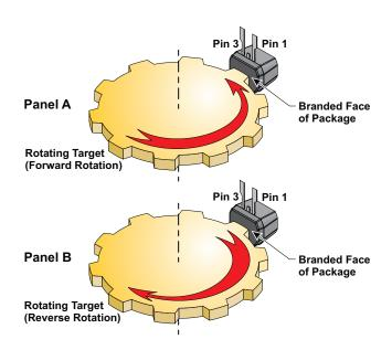
Figure 4: Target Rotation ("F" Variant Shown)
