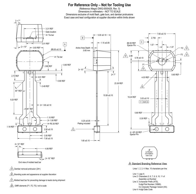
Figure 9: Package SN, 3-Pin SIP
