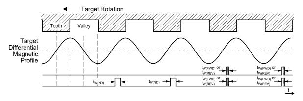
Figure 5: Output options after power-on
