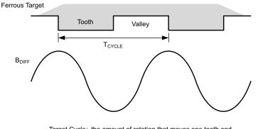
T<sub>CYCLE</sub> = Target Cycle; the amount of rotation that moves one tooth and valley across the sensor.
